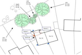
Crack monitoring has been undertaken, but as if to illustrate the problems with this technique, studs fell off from two of the stations, and readings are at uneven intervals - see following page.
