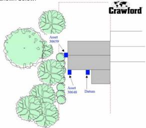
The installation was undertaken in March 2009 and the objective is understanding the amount of movement we will see on Boulder Clay. Our geology model suggests a very low P.I. - around 10 - 15% taking account of percentage passing. Barely a shrinkable commodity.
