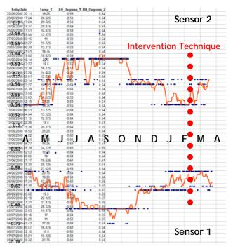
The red lines plots a 6 Interval Moving Average used to reduce signal fluctuations
