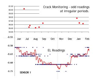
Crack monitoring (upper of the two graphs) tells us there is enhanced periodic movement that implicates the tree, but we can hardly take comfort in delivering this level of service when an alternative technology, costing little more, delivering objective data at regular intervals, is available. Graeme Phipps from SPPS was testing the telemetry device for measuring cracks at Aldenham, and provided the following output from 2007 and 2008.
